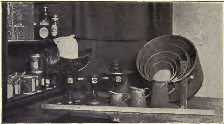
TEST SET OF WEIGHTS AND MEASURES RECOMMENDED BY THE U. S. BUREAU OF STANDARDS
